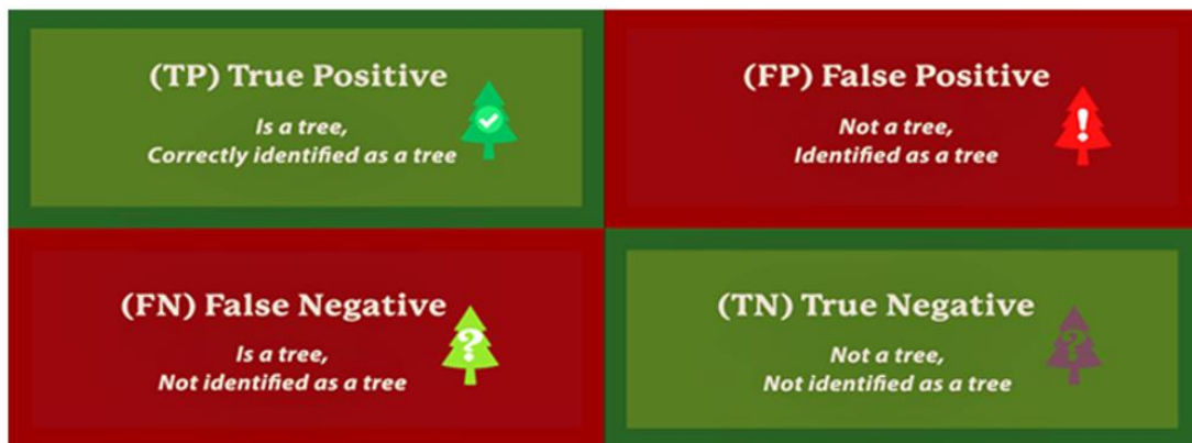
Figure 7. Explanation of a confusion matrix created for seedling detection.
