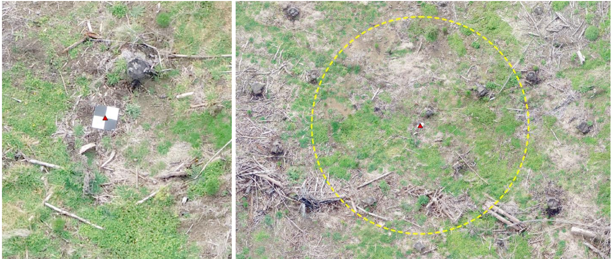
Figure 5. Examples of orthomosaics in which the plot centre has been manually annotated (red triangle) in ArcGIS Pro, and a circular buffer (yellow) added demarcating the plot boundary.
