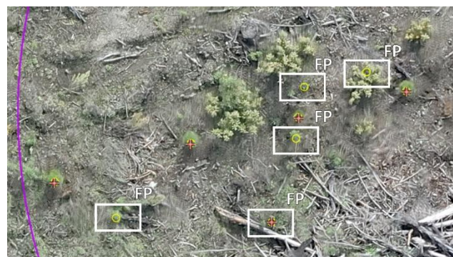
Figure 4. Examples of FPs (white boxes) in plot 4. Detections are represented by yellow circles (0.7 cm data) and red crosses (1 cm data).
